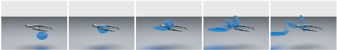
Figure 1: A ball of water collides with a skeleton hand. The frames in this animation were efficiently computed using our technique: the ball and the splashes belonged to domains that were merged and split to minimize computation cells.
